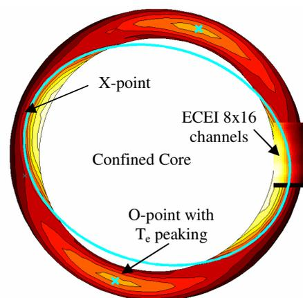
*ECE-Imaging measurement of island with temperature peaking (frame of movie)*
